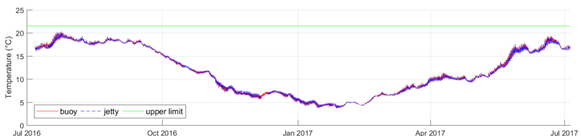
Figure 10. Annual time series of water temperature measured by the buoy and jetty system. The green line indicates the limiting threshold defined in the AMEP Development Consent Order (being water temperature must not reach 21.5^{\circ}\text{C} ).
